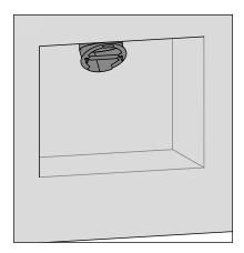
Install the flexible or solid flue so that is comes out close to where the appliance outlet will be located. Attach the smoke outlet connection provided with the fireplace (if using a flexi flue, use a metal duct clamp - not provided).
